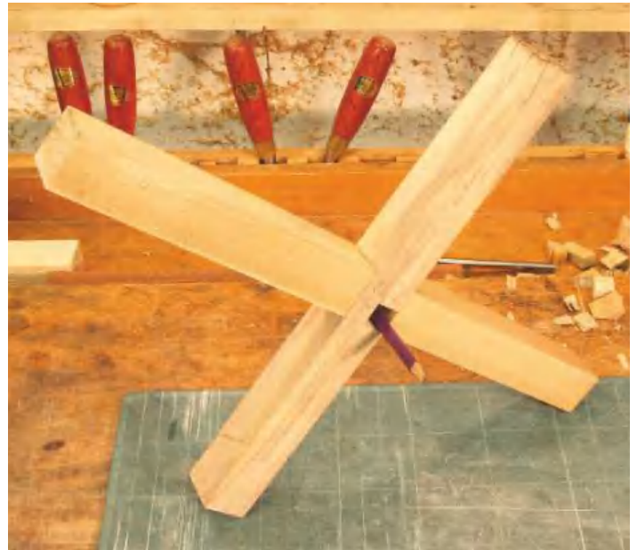
▲ Pic.10 After removal of the next group of squares, they fully interlock and leave an aligned void on each piece. I have pushed a pencil through these voids to show where they are
